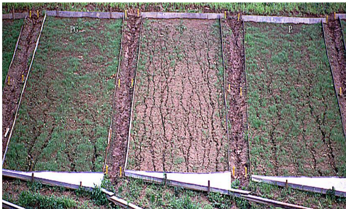
Figure 6. Photograph of three representative plots at the RDF natural rainfall site with treatments (left to right) of PAM and gypsum (PG), control (C), and PAM (P). This picture was taken on 19 June 1998, three weeks after seeding. Intense storms produced 130 mm of rainfall during this three-week period. Notice the reduced rilling and improved grass growth on the treated plots.
