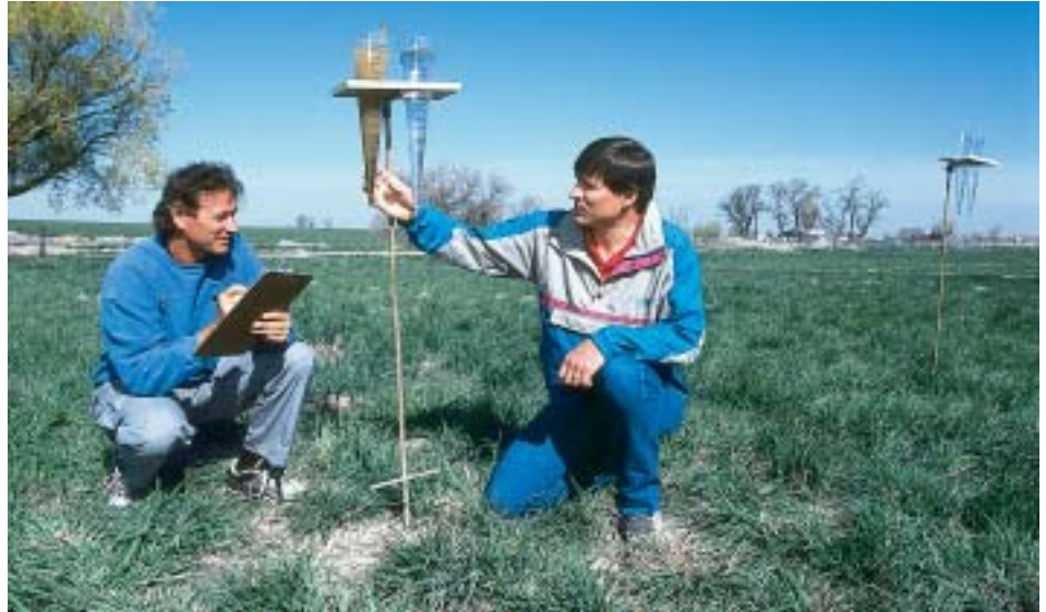
Jim Entry (left) and Dave Bjorneberg record sediment concentrations from furrow irrigation runoff samples. The darker sample on the left is from an untreated furrow.
